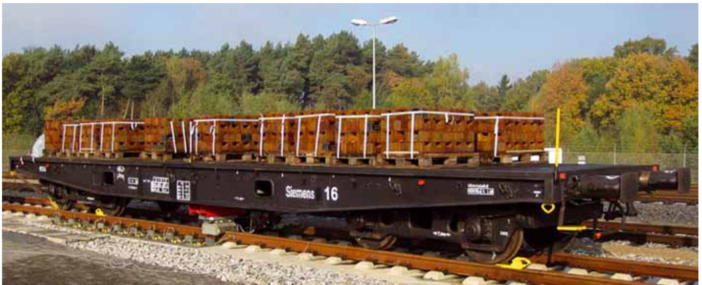
Fig. 8: Loaded Smp flat car with calibration device
