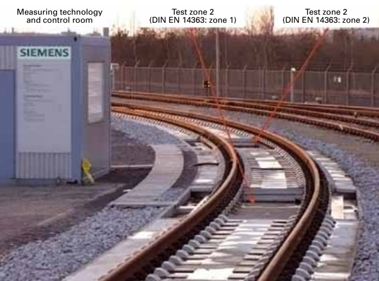
Fig. 4: View of measuring track curve
