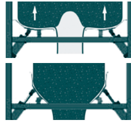
Full Bulk Bag – vertical agitation breaks material bridging.
