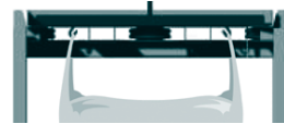
Four pneumatic cylinders lift the bag-lifting frame simultaneously to fully extend the Bulk Bag.
